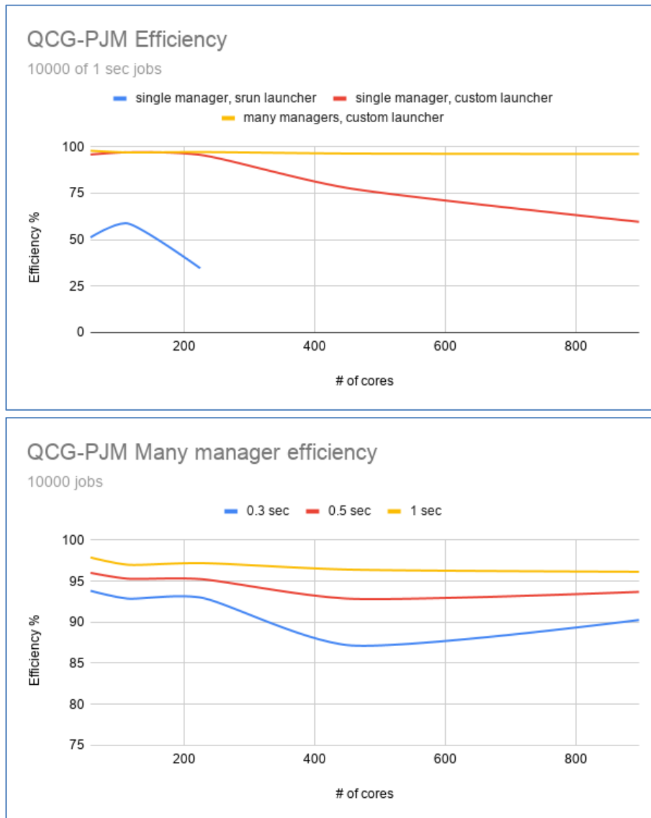
Figure 5 - Comparison of efficiency of different versions of QCG Pilot Job Manager
